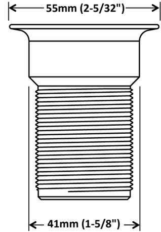
Only install these two for thin-sink applications (e.g. metal sinks or sink thickness  $\leq 1/2'' \pm$ )
