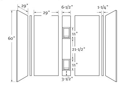
Designed to fit tub area 30" deep x 60" wide (762 mm x 1524 mm), or smaller
